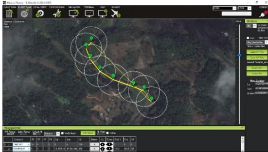
Figure 9 UAV Flight Plan using Mavlink Mission Planner
