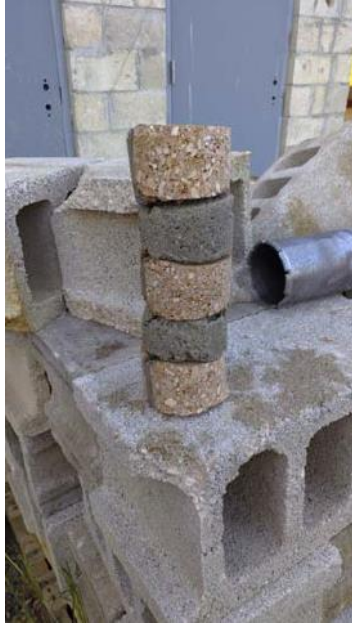
Figure 2 Core taken during Additional Field Testing
