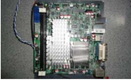
Figure 2 Front View of a LittleFE® Cluster Board
