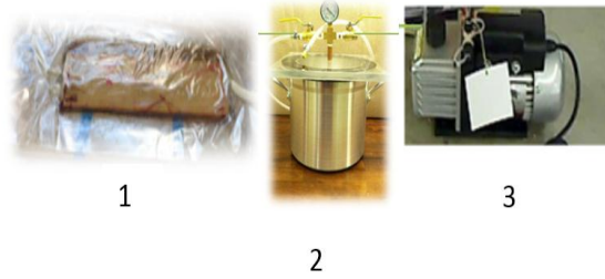
Figure 6 Vacuum Process 1 Blade Covered, 2 Vacuum Chamber and 3 Vacuum Centrifugal Pump
