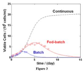
Graph illustrating how is the performance of Batch, Fed-Batch and Continuous processing achieving the required cell density. Perfusion was designed as a Continuous processing.
