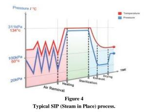
For the three phases that compose the sterilization cycles (Pre-Conditioning, Exposure and Post-Conditioning), six factors are particularly critical to assure successful steam sterilization: Time, Temperature. Moisture, Direct steam contact, Air removal and Drying [3].
