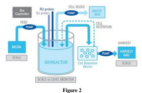
Typical Perfusion process in bio-reactors
