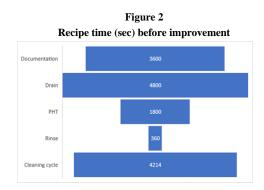
The data included in the figure above have the consumption time of each stage. If the chart was studied, many stages are repetitive. The total time of each stage were evaluated and consolidated in the project to reduce the cycle time of the cleaning recipe. Each stage was consulted with the validation personnel to determine the critical step of the recipe and they confirmed that no step can be eliminated, but can be consolidated.
