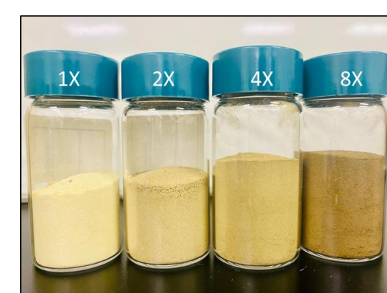
Figure 3. Ni-CN prepared with different amount of nickel chloride. X = grams of the nickel chloride used in the synthesis.
