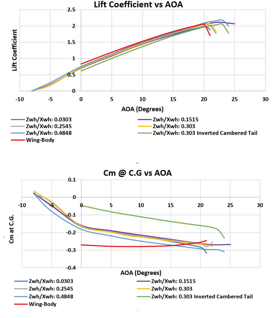
The new method of downwash predicts the AC by a minimum and maximum difference of 1.26% and 11.7% respectively. A special case combining XFRL5 and new downwash law method, to calculate the AC and longitudinal stability. This hybrid method and shows an AC
