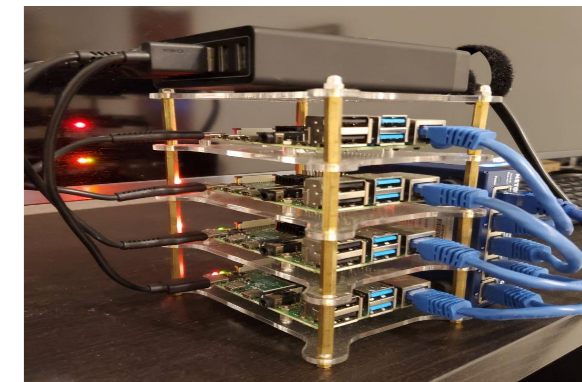
Figure 8: Image of Raspberry Pi Cluster used in project.
