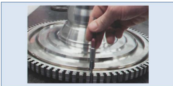
Figure 4 Disk Inspection – Calibrated Pin Checks
