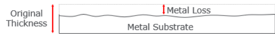
Figure 5 General Corrosion Example (A small amount of metal is taken evenly throughout the system or coupon)
