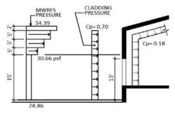
Figure 8 - Pressure Profile as ASCE
