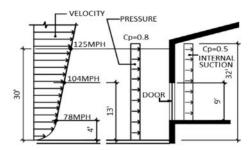
Figure 7 - Wind Velocity and Pressure
