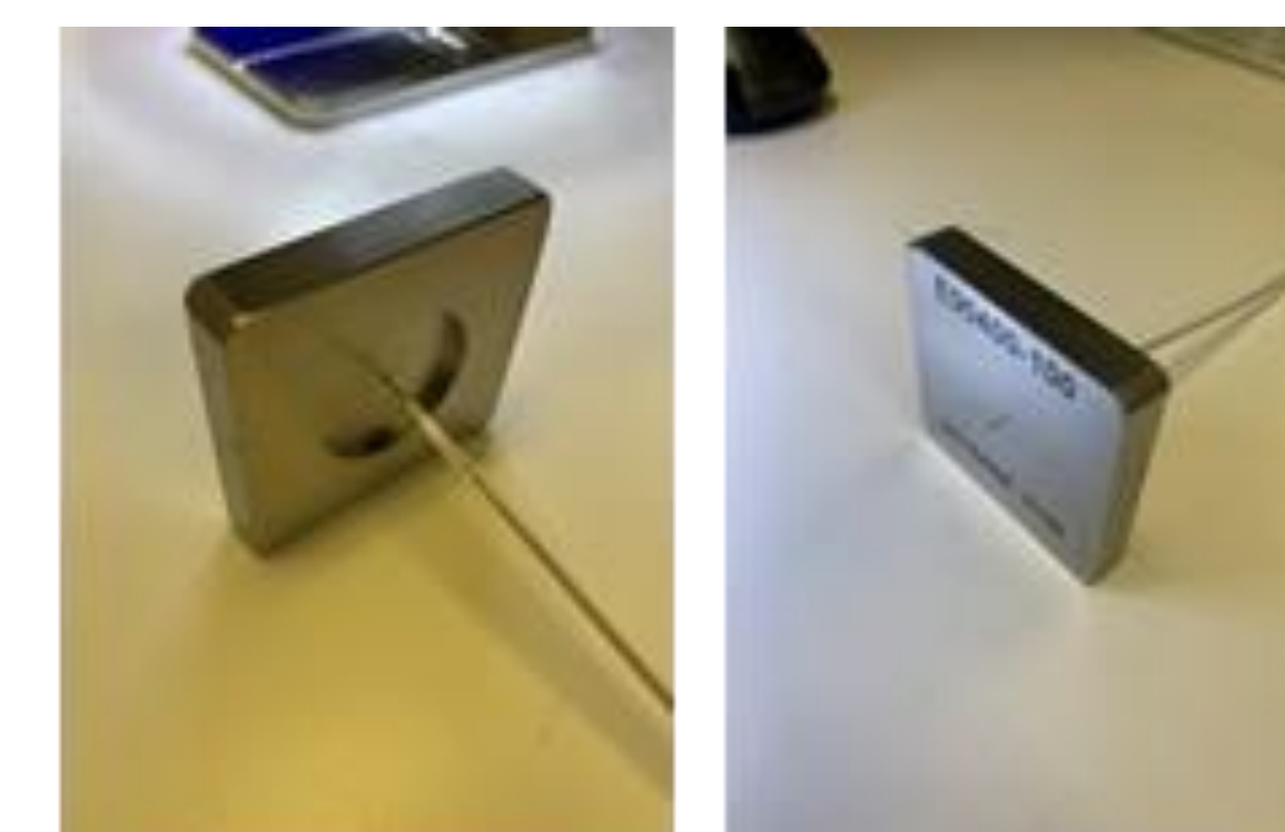
Figure 5 Inspection of the center cable by the Go/No Go Gauge
