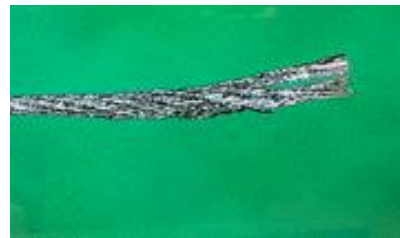
Figure 3 Center Cable Fray Defect
