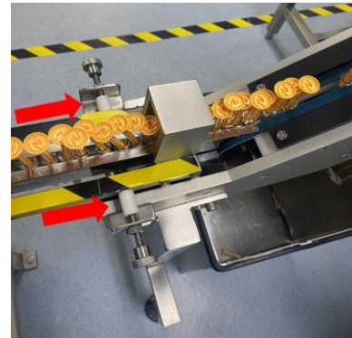
Figure 3 Vibratory Rail Support Mechanism
