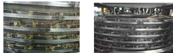
Figure 14 Before and After the Sensor was installed on the Bowl Feeder.
