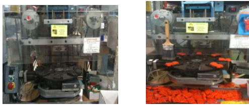
Figure 12 Before and After stalling the brush on painting top station.
