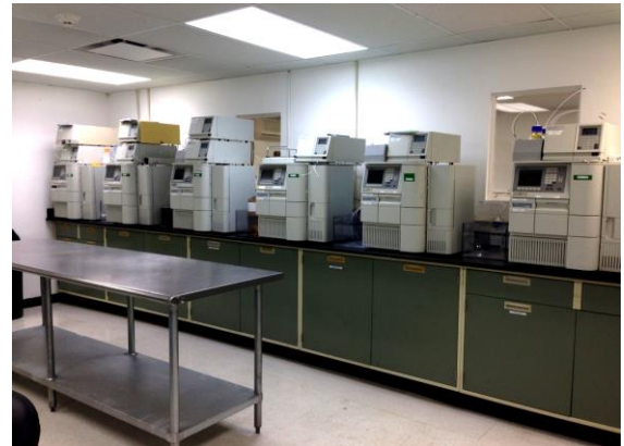
After Improvement Top benches installed to maximize HPLC capacity and providing space for storage and waste disposal.
