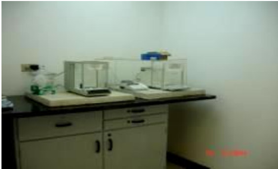
Before Improvement Unstable balances due to inadequate supporting bench
