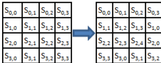
Figure 15 Shift Row Transformation
