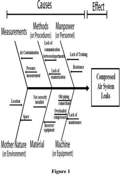
Fishbone Diagram of the Compressed Air Leaks
